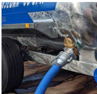
Side gate valve
