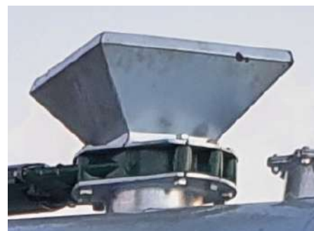
Upper gate valve
