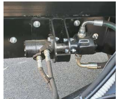
Tipping with hydraulic motor and pump
