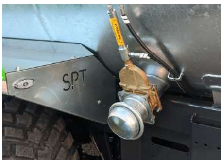
Hydraulic side gate valve
