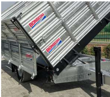
Side walls opening upside down
