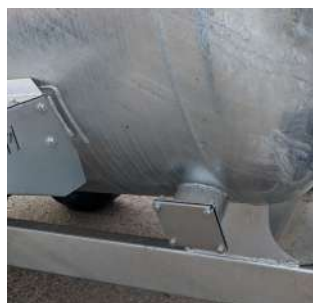
Side gate valve arrangement
