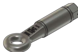
STANDARD EYE up to 6 t. hole diam. 35 mm up to 14 t. hole diam. 50 mm up to 20 t. hole diam. 76 mm (capacity up to 3000 kg)
